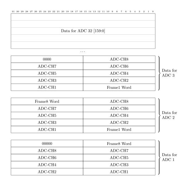
Figure 3: Frame word: the FIRST bit is 0 for non-first samples, and 1 for BCR asserted (and BCID is 0). Data word: the OVER bit is set to 1 for ADC overflow.
