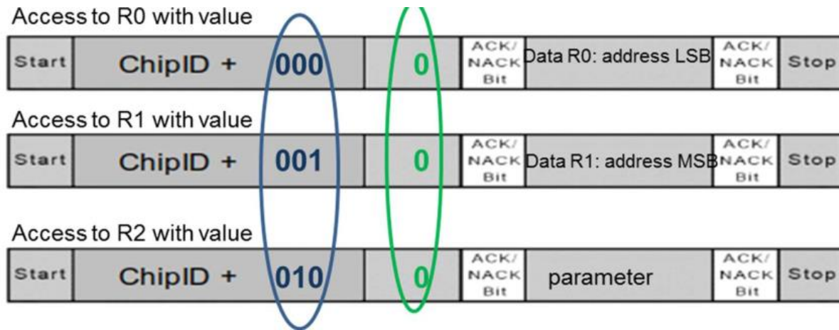
Figure 1: I2C sequence to write one SC register.
