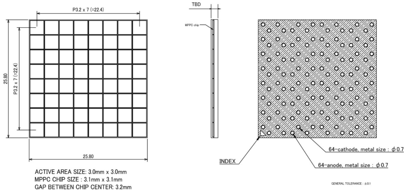
**S12642-1616PA-50 (3x3mm<sup>2</sup>, 16x16ch, 256ch, p50μm)**
