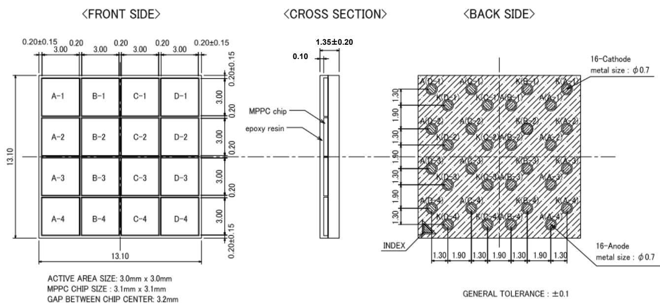
**S12642-0808PA-50 (3x3mm<sup>2</sup>, 8x8ch, 64ch, p50μm)**
