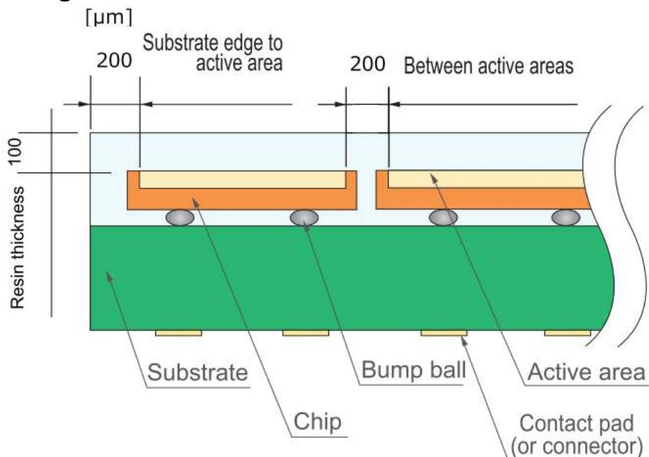
**■ Dimensional outline** (unit: mm, Tolerance:  $\pm 0.1$  mm unless otherwise noted)**S12642-0404PA-50 (3x3mm<sup>2</sup>, 4x4ch, 16ch, p50μm)**
