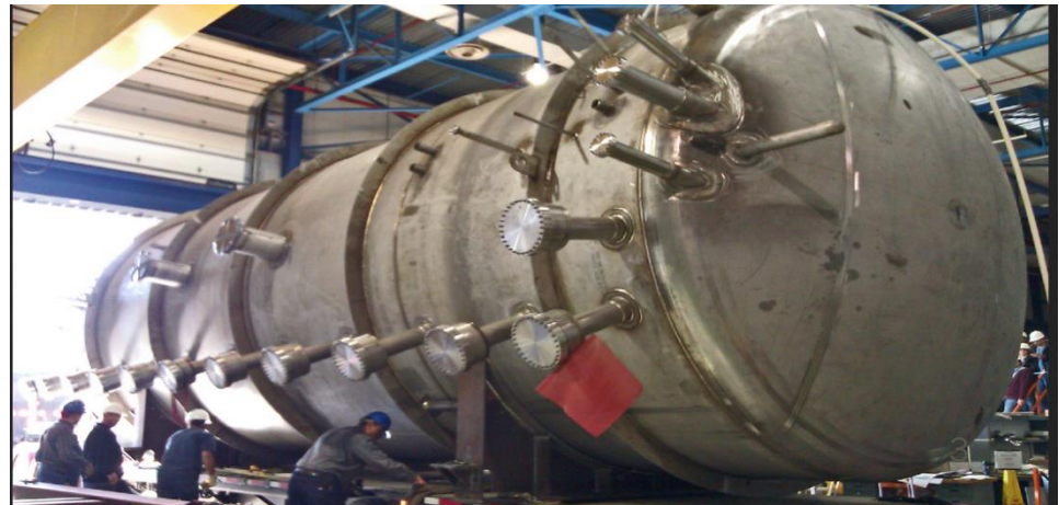
Cryostat During Delivery
