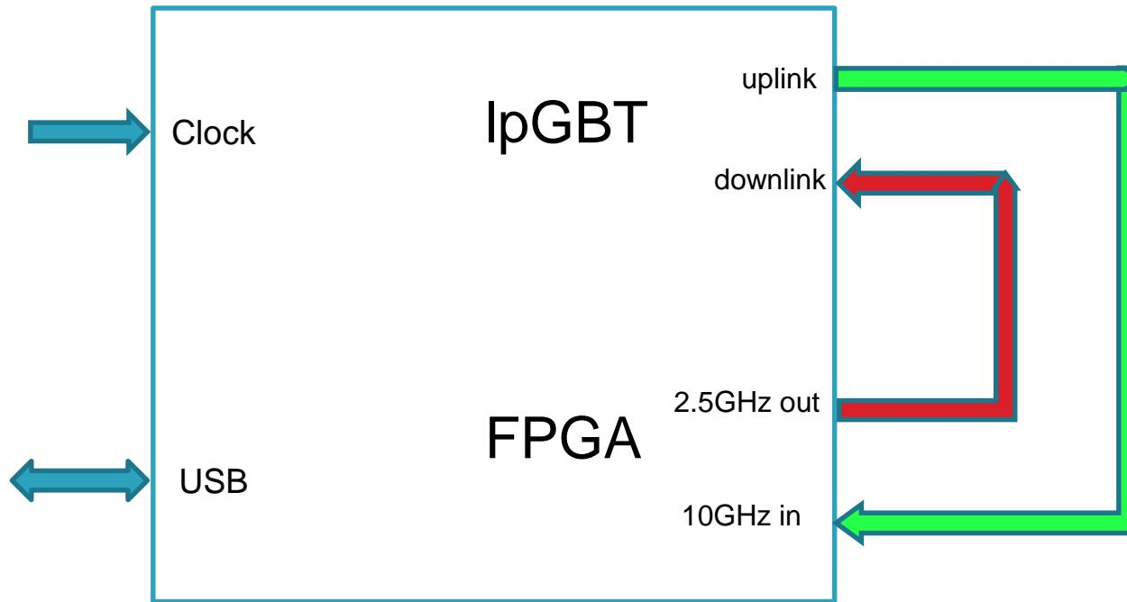
With `LOCKMODE==1'b1`, `MODE[3:0]==10Gbps/FEC5/Transceiver` and working IC/EC channels:
