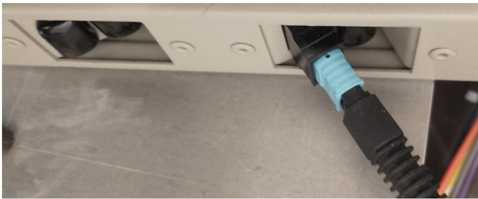
The fiber MPO-MPO cable is connected to the FELIX card as shown here:
