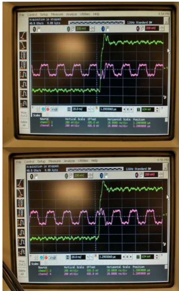
SCOPE Traces of SCL + CP40N/P for I2C Write Command to Board 503 COLUTA 14 NO ACK
